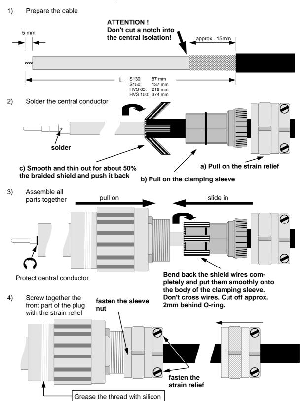
This mounting instruction is also valid logically for connectors of the same construction e.g. S130, HVS 65, HVS 100 or HVS 150. The difference is only in the length of the plug and in the cable diameter.
