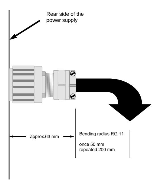
Bending radius other cables once repeated C 2124 150 mm approx. 4x C 2121 220 mm approx. 4x
